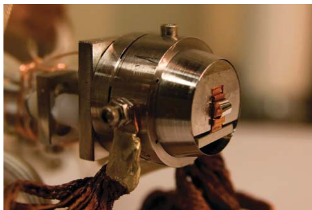
Fig. 1 Pyroelectric heat detector and its holder. The 4 mm-wide pyroelectric polymer ribbon, in the form of an arch, protrudes from this conical holder designed to fit exactly into the conical recess in the mating sample holder for the single crystal, so that the flexible ribbon compresses against the back surface of the crystal, deforming inward by a fixed amount ( \sim 2 \text{ mm} ) and simultaneously flattening across the crystal's surface. This holder is cooled by Cu braids which attach to a gas-cooled Cu reservoir, and can be stabilized at temperatures down to 100 K. It is retracted from the sample holder (by translating to the left), so that the sample holder can be moved to different parts of the chamber for surface analysis, cleaning or annealing.
